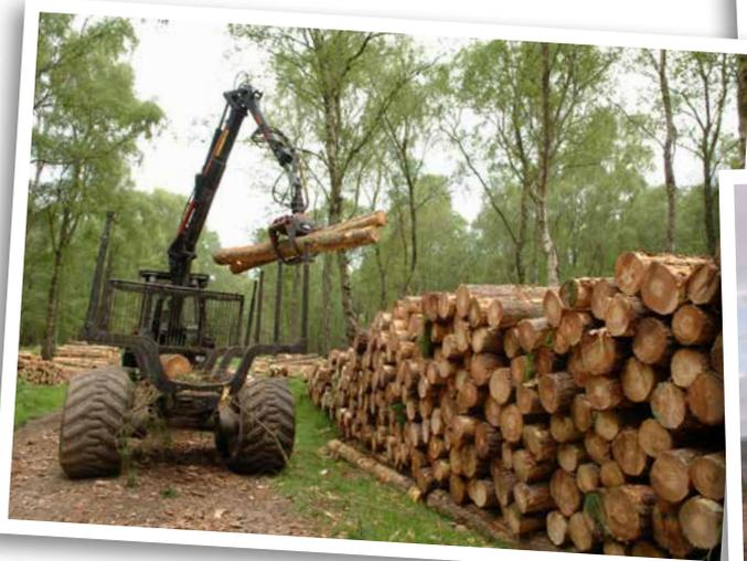
Forwarder – stacking logs at roadside
